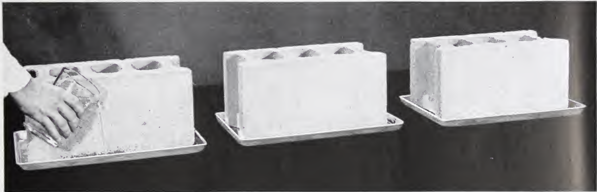
Three concrete blocks—left made with regular cement, center with Medusa Waterproofed Gray Portland Cement and right with Medusa Concentrated Waterproofing Paste—were placed in pans which were filled with water.
